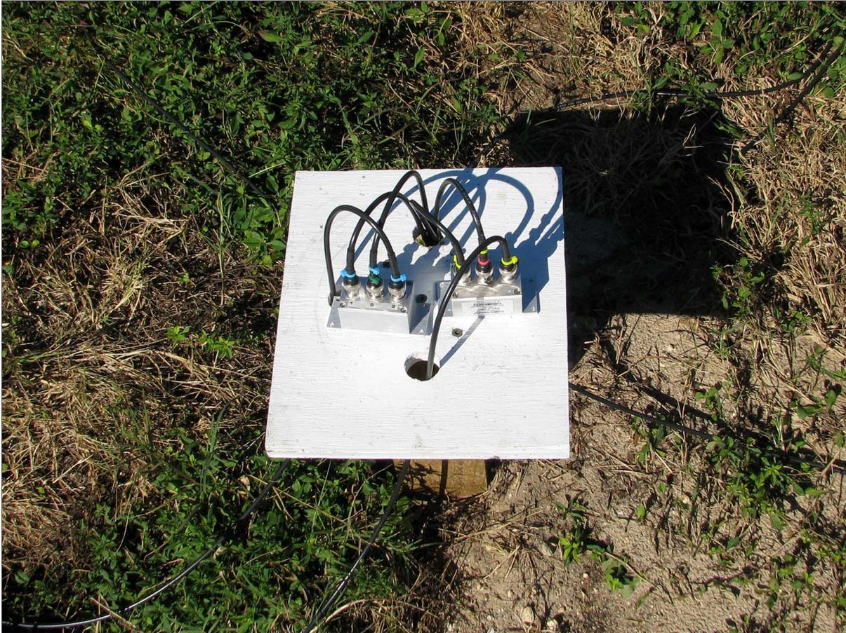
Here is the inside of one of the three junction boxes used in the TFD array. This one contains the two power combiners that bring signals from the two squares together, for transmission to the receivers. There are no delay cables installed in this picture, so the beam was pointing at zenith.
