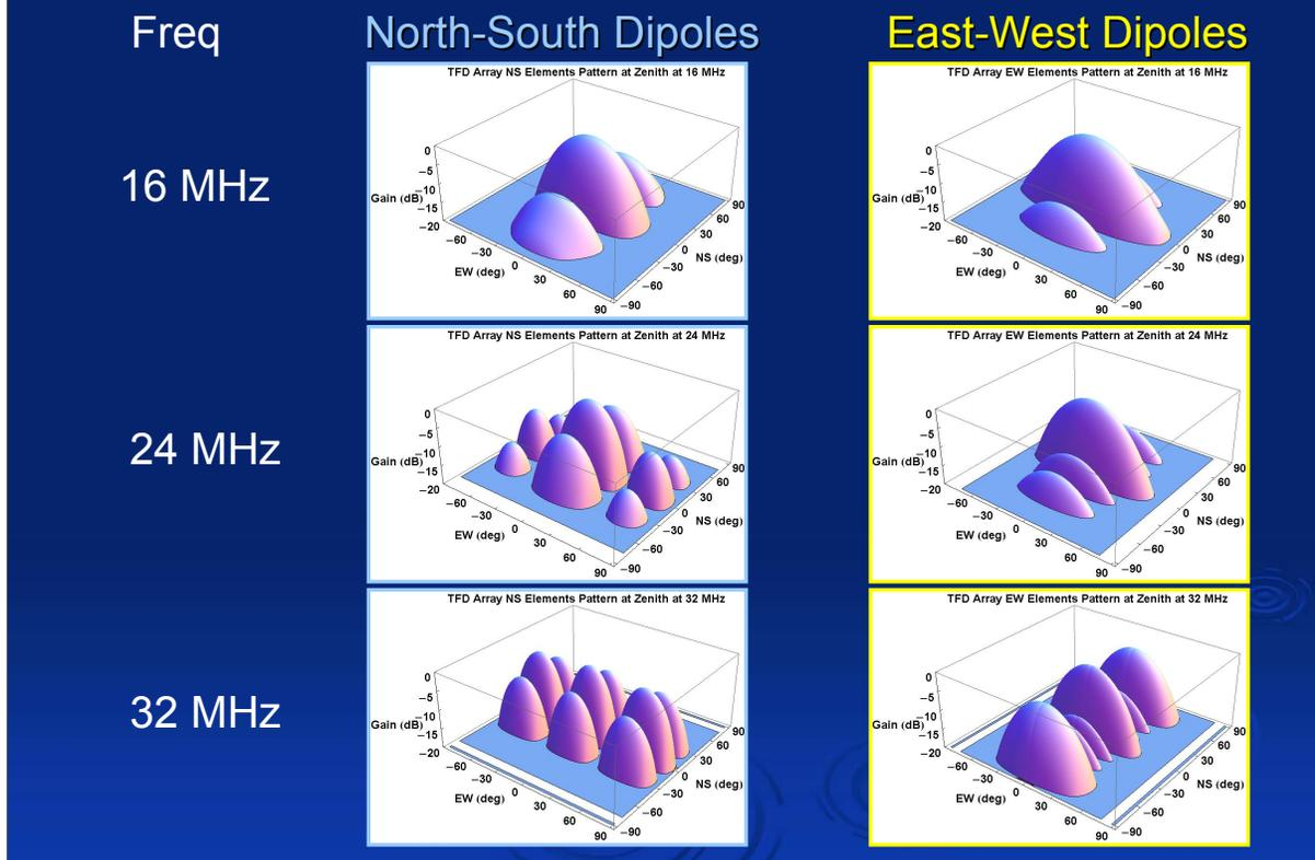
And here are the real beams (array steered to zenith), found by simply multiplying the array factors by the element Factors. This is **much** easier than running the electromagnetic field calculations for eight real TFD antennas spaced 32 feet apart in a rectangular array.
