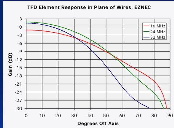
Here are rectangular plots of one TFD element's response (elevation patterns) in two directions: in the plane broadside to the element's wires and in the plane of the element's wires. Plot traces represent the elevation patterns at 16, 24, and 32 MHz.
