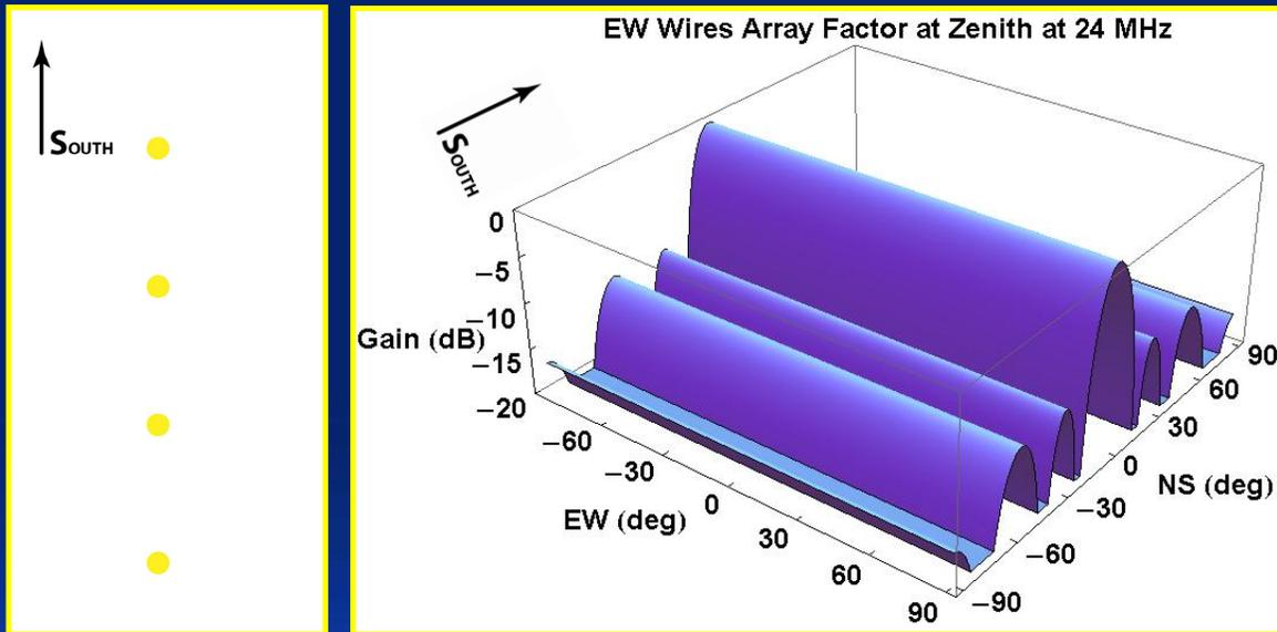
An array factor is the beam one would get by replacing the real array elements with **isotropic radiators**. Since isotropic radiators receive equally well from all directions, calculation of the beam is relatively easy (see slide # 46) – it is simply an interference pattern.
