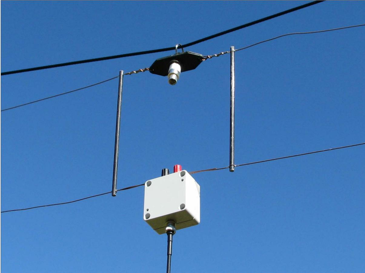
A Budwig center insulator allows for a center support rope to hold up the middle of the element. It is also the attachment point for the 800 ohm non-inductive terminating resistor, which is soldered inside a PL-259 coax connector.
