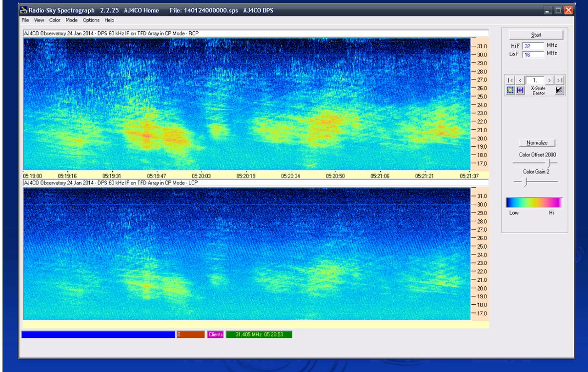
The DPS hardware is controlled by the Radio Sky Spectrograph (RSS) software. Jim Sky, who graciously makes RSS available to all for free, made several modifications to RSS to allow it to control the DPS, record two correlated spectral data streams, and display two waterfalls in real time.
