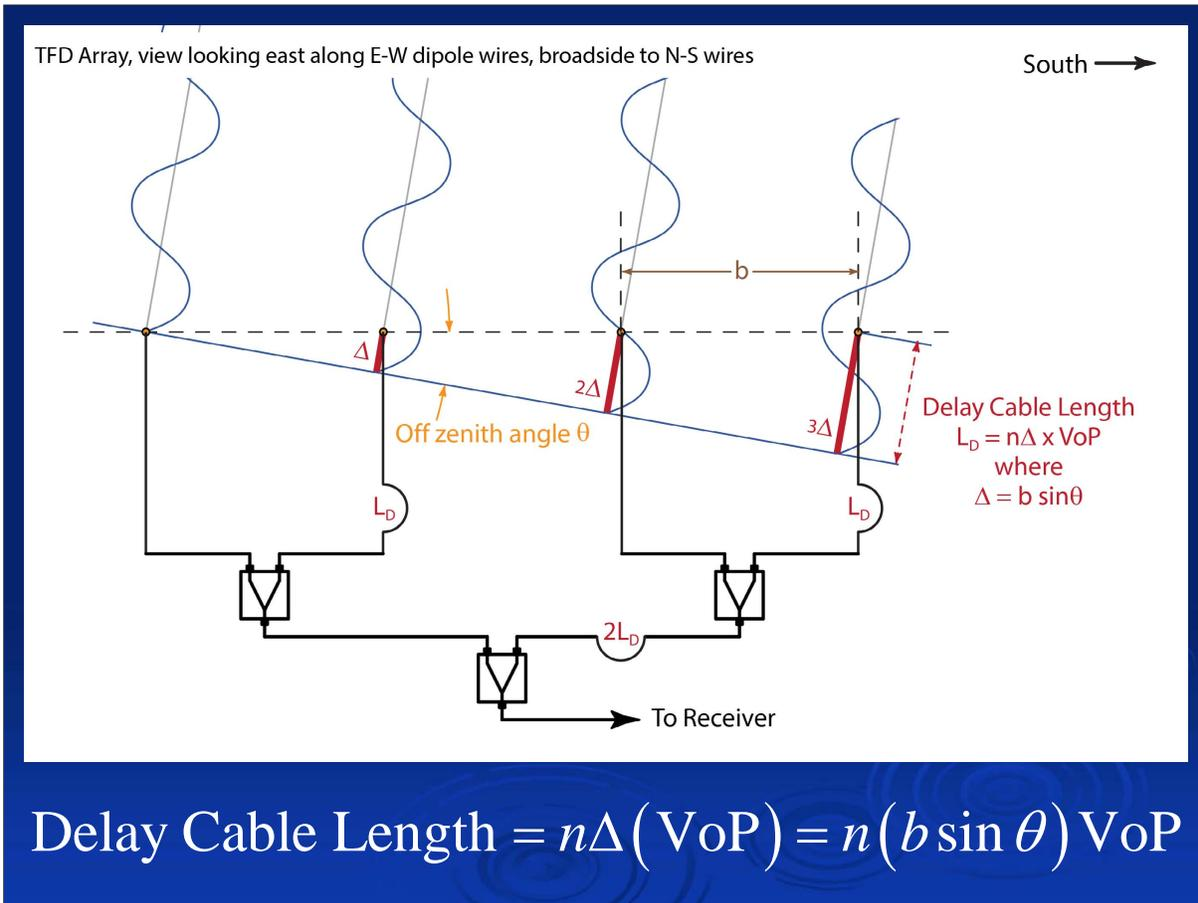
Here is an example of an array with more elements. The process is exactly the same as described on the previous slide, just with multiple delay cables.
