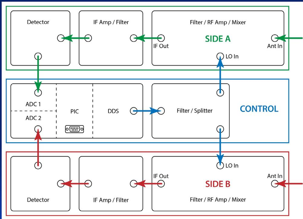
The design is basically two FSX spectrographs (as discussed in the Advanced Systems talk) tied together with a common DDS LO and controlled by a single PIC. The ADC's of each side are triggered simultaneously. The samples from the ADC in each "side" of the DPS are thus correlated, making it possible to obtain meaningful results from mathematical operations on the samples from each side (cross polarization ratio and total power).
