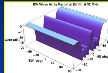
Here are the array factors for three frequencies. This represents the interference pattern formed by **isotropic radiators** in place of the real TFD elements of the array.
