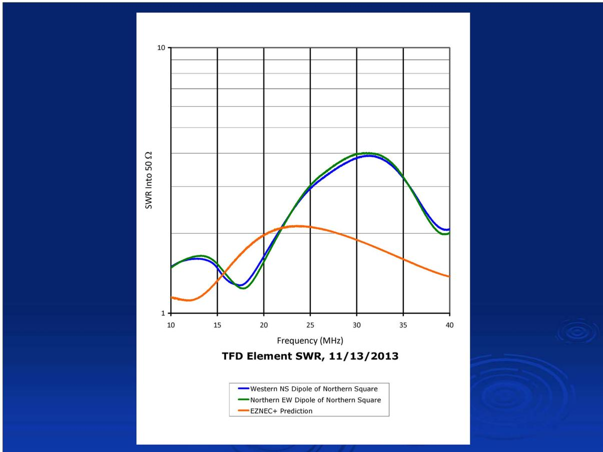
SWR sweeps performed with a VNA-2180 on two different single TFD elements (green & blue) at their balun outputs as installed in the 8-element array, compared to the EZNEC prediction for a single TFD element (orange) by itself over ground.
