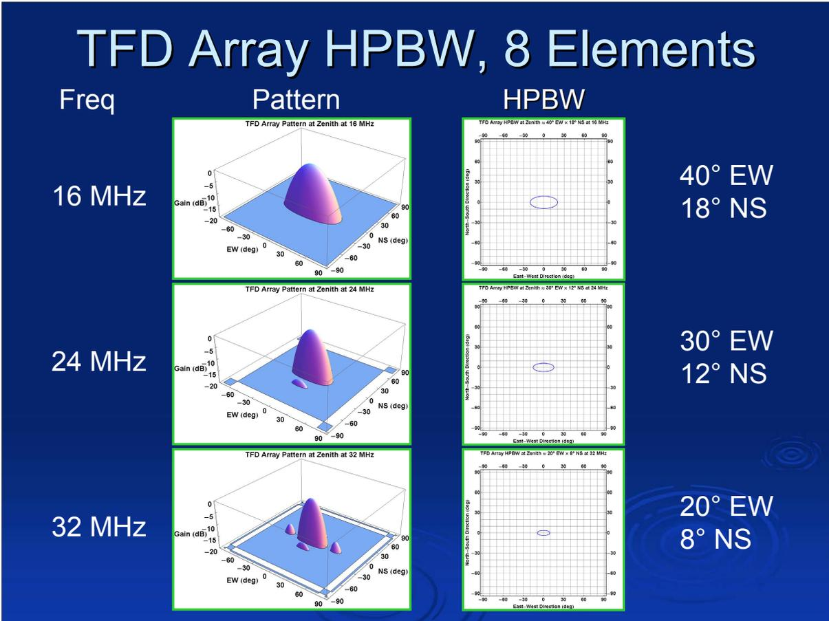
Plots are for a **beam at zenith** (no delay cables). That is, these beams represent the yellow and blue arrays multiplied together.
