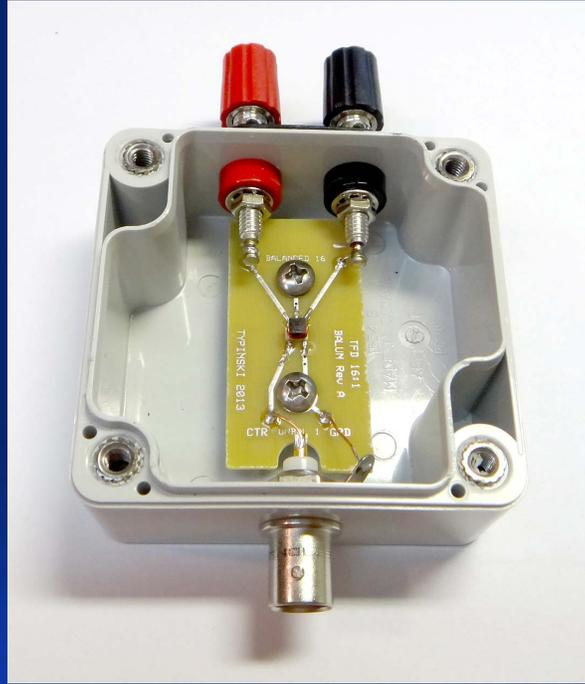
The balun is custom designed and built around a Mini-Circuits TC16-161TX+ 16:1 SMD balun transformer. The unit is rated at 250 mW; so far, lightning spikes have not damaged any of the TFD's baluns.
