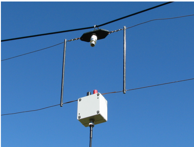
Figure 4 – Center of TFD element. View looking north. Note that the positive (red) terminal is on the east side. This could also be looking east with the positive (red) terminal on the south side.
