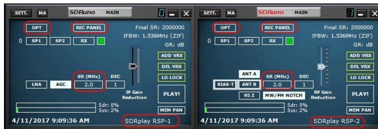
(Left: RSP-1 Right: RSP-2/2PRO (RSP2/RSP2pro has antenna port and MW/FM notch filter selection options)
