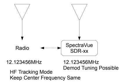
• HF Tracking, Allow independent tuning within HF band
