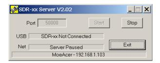
2. Connect the SDR-xx USB cable to the remote PC and apply power to the SDR-xx if required. The server should connect to the SDR-xx and the following status should result.
