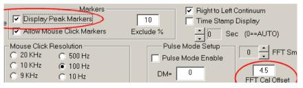
In the direct input mode of the SDR-14, a value of 4.5dB will be very close since this is the level in dBm where the A/D begins to clip. If the internal preamp or an external one is used, then one must change the value accordingly.
