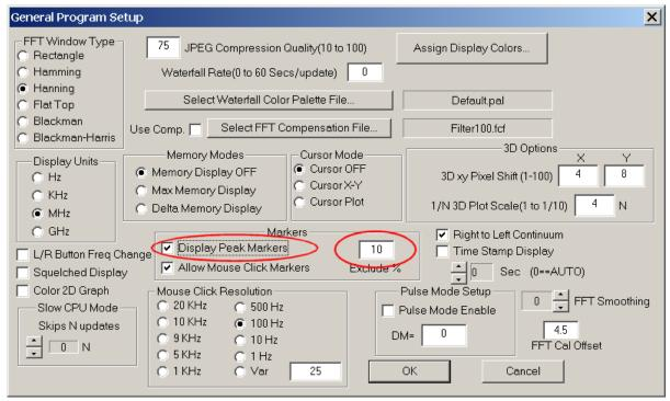
3. Setup the main screen as follows with an FFT size of 65536, an average of 5 or so, a center frequency of 10MHz(for WWV), demod OFF, and a span of 500Hz. Press Start and adjust the screen to allow easy viewing of the 10MHz peak. Note the little red mark on the peak and its corresponding marker frequency of 9.9999979Mhz in the status bar. This is the measured frequency of WWV and shows that the program is off by about 3Hz.
