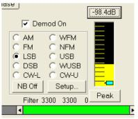
The "Demod On" checkbox enables or disables the demodulator section. It is only available when the SDR-xx bandwidth is within certain ranges.
