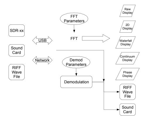
SpectraVue takes as input sources a variety of SDR-xx Software Defined Receivers from RFSpace, A PC Sound Card, or RIFF .wav file. The FFT (Fast Fourier Transform) is a math transform that converts the time domain data input samples into frequency domain data that is used for various display modes that show signal power versus frequency. SpectraVue can also perform simple demodulation operations and output the audio to the sound card or a .wav file.
