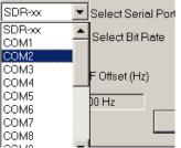
The Select Serial Port menu selects the desired PC COMx port if you wish to use a PC COM port. The SDR-xx selection can be used to select the built in serial port of the SDR instead of the PC COM port. Not all models have this capability.
