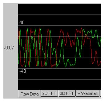
If it is real data then there is only one trace. Complex data is displayed as two different traces with different colors. The two numbers in the display area are the max and min values of the incoming signal. The range of inputs is a 16-bit value or 0 to +/- 32767.
