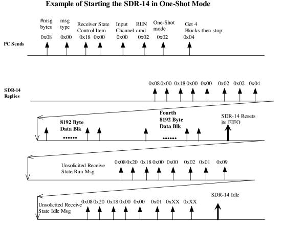
SDR-14 begins sending data messages back to PC until the 4th block is sent, It then resets its FIFO, then sends an Unsolicited Run Receive State Msg and an Unsolicited Run Receive State Msg then stops and goes idle.
