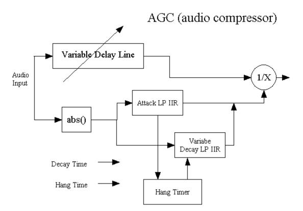
The demodulator AGC uses a simple audio compressor scheme with variable decay filters and also a hang timer.
