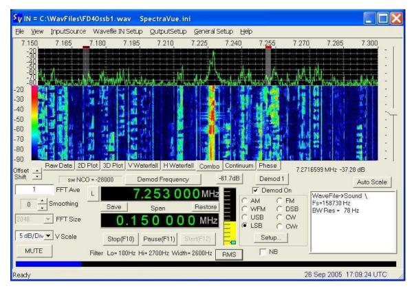
Across the top of the screen are menu buttons that are used to setup the majority of all the program settings.
