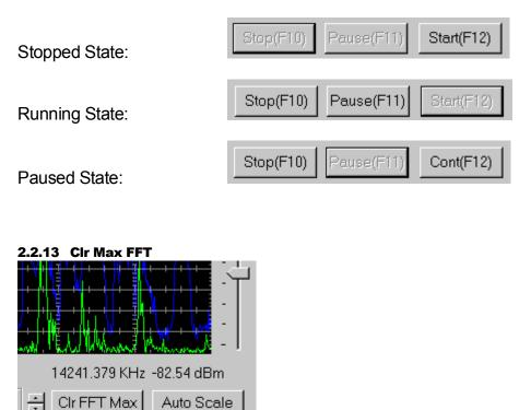
This button is used to reset the max hold buffer when the maximum hold display is active.
