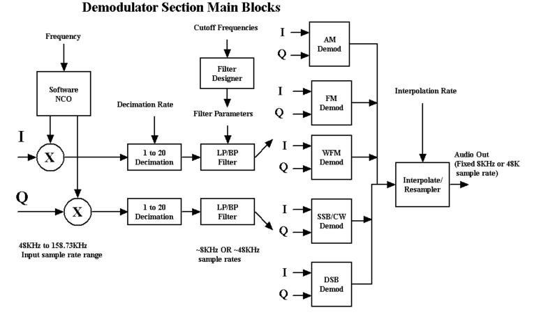
I/Q data from the input source is sent to the demodulator block. It is first "tuned" to the desired signal using a complex mixer and software NCO. This allows one to tune in signals anywhere within the input bandwidth which could be up to 150KHz wide..
