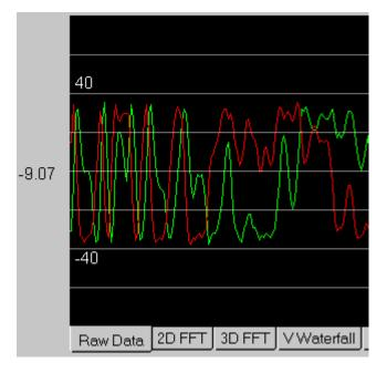
If it is real data then there is only one trace. Complex data is displayed as two different traces with different colors. The two numbers in the display area are the max and min values of the incoming signal. The range of inputs is a 16-bit value or 0 to  $\pm$  32767.
