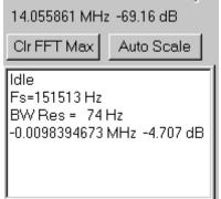
This text box displays the program status as well as some information on current sample rates and FFT resolutions.
