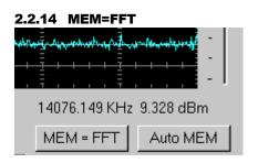
This button is used to store the current FFT display into the reference buffer when the delta FFT mode is active.
