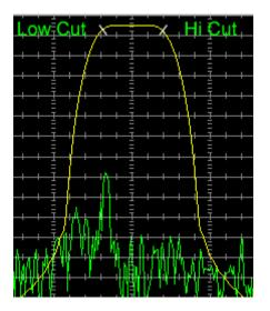
If the high cut off is greater than 3600Hz, then a higher sample rate is used in the filters. This causes a jump in the shape of filters about this transition point. The higher cutoff filters are not as sharp as the narrower ones.
