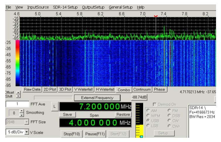
The Button above the main frequency control allows toggling the frequency control between the SDRxx center frequency and the External Radio center frequency. The white marker on the display shows where the external radio is tuned.
