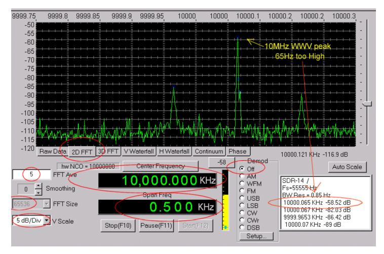
4. Stop the capturing and open the SDR-xx Setup menu. Notice the measured frequency has been automatically placed in the box(if you had peak markers checked and it was marking the correct reference peak) One can manually enter the Reference and Meas frequencies if not using a 10MHz reference.
