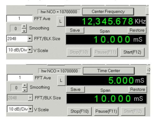
This mode is not useful at the present time with the current hardware/firmware due to the lack of triggering capability on the current SDR-xx hardware and firmware versions. Later releases may incorporate triggering to utilize this mode.
