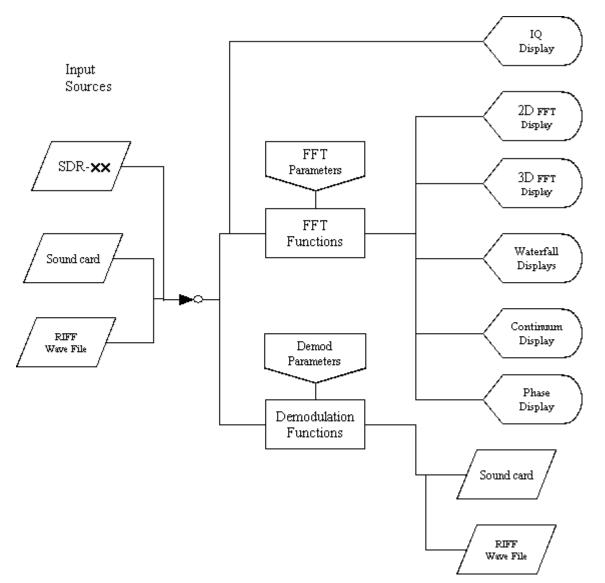
The data input can come from the an SDR-xx unit, a soundcard, or a RIFF .wav file.
