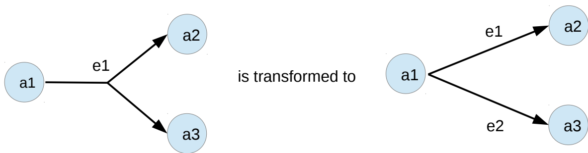
Fig. 4. On this figure you could see how the multi destination edge is transformed into two separate edges in order to have a regular directed graph.
