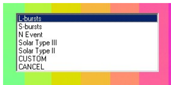
Illustration 29: The customizable Annotate pop-up menu is accessed by right clicking on a loaded spectrogram and selecting Annotate or Annotate Region.
