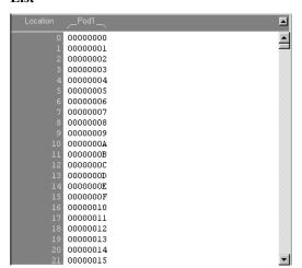
A List display provides a non-graphical list of data on the screen. Scroll bars allow the user to navigate to different parts of the data.
