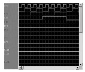
Digital display provides a graphical representation of data on the screen. A state or timing diagram is displayed for each of the bits in the pattern.
