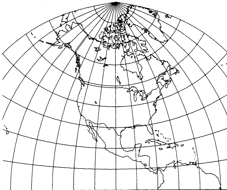
FIGURE 25.—North America on a Polyconic projection grid, central meridian long. 100° W., using a 10° interval. The parallels are arcs of circles which are not concentric, but have radii equal to the radius of curvature of the parallel at the Earth's surface. The meridians are complex curves formed by connecting points marked off along the parallels at their true distances. Used by the USGS for topographic quadrangle maps.
