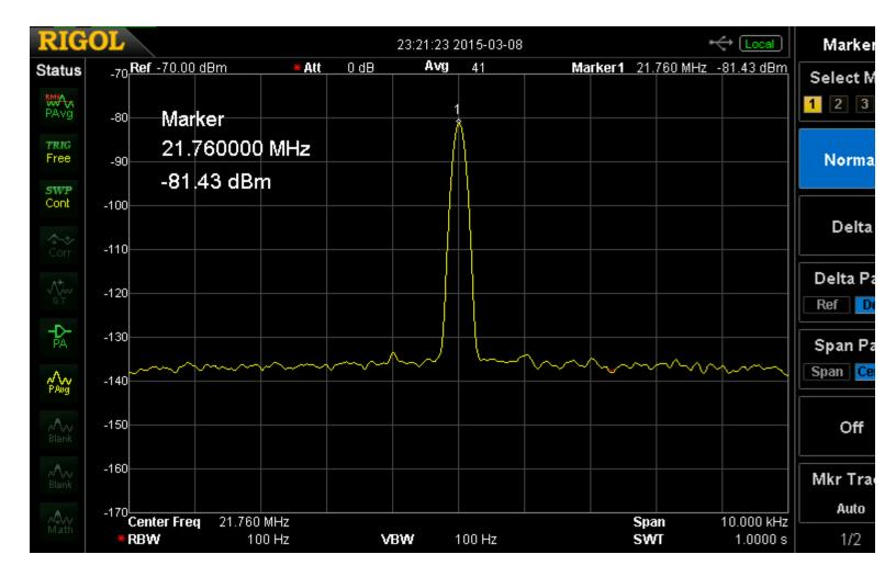
Results: 120.2 - 81.4 ---> cross polarization leakage in the hybrid is 38.8 dB down.
