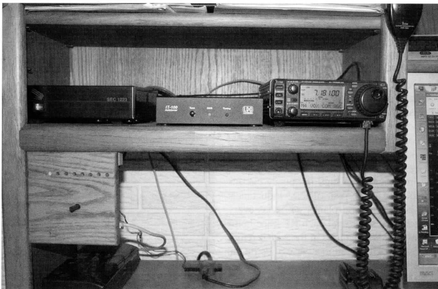
Figure 2 — This photo of my operating position shows my power supply, LDG Autotuner, and Icom IC-706 MKIIG radio. The antenna selector control panel is mounted behind a block of wood to match the operating position shelf. You can see the selector shaft, with the first of eight LEDs illuminated to show which antenna has been selected. I still have to add labels below the LEDs to help identify the antennas.
