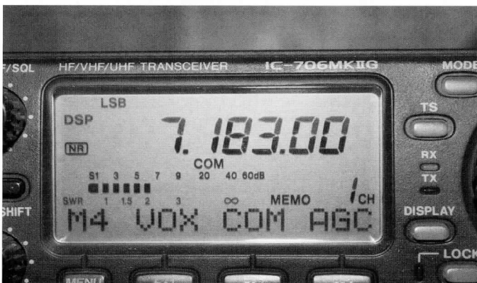
Figure 3 — Here is a close-up of the Icom radio display. Notice that with a 40 m antenna connected, the S meter is showing an S6 signal.
