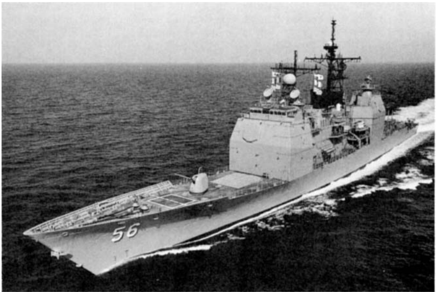
FIG. 7.1 Guided missile cruiser showing two out of four phased array antennas. (Courtesy of Ingalls Shipbuilding Division of Litton.)
