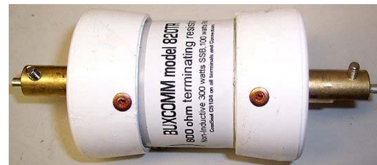
Photo 1: With the standard BUXCOMM T2FD, 300 watt antennas, we make the characteristic impedance of the BUXCOMM balanced termination, folded dipole 600 Ohms using the BUXCOMM model BTR600. Matching the pair, we use the BUXCOMM MM161 BALUN.
