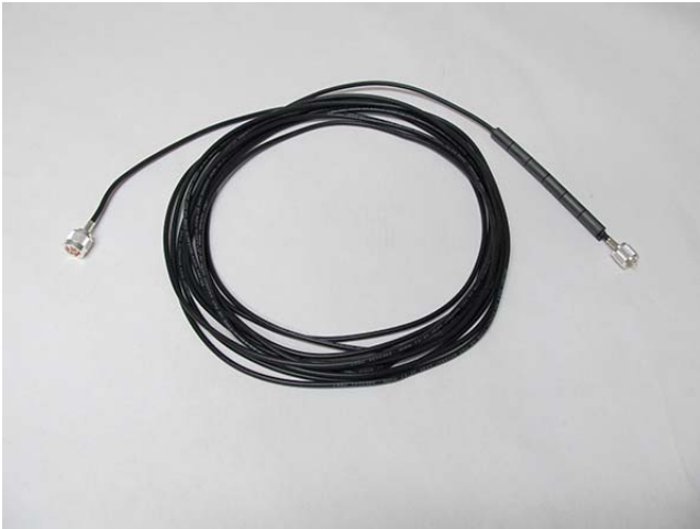
One piece of RG-58 (Belden 8259) cut to one wavelength long. The feed point end has a PL-259 crimp connector after six ferrite beads that form a common mode choke to act as a balun. These inexpensive toroids, Fair-Rite P/N 2631480002 available from Mouser, fit snugly on the RG-58. The far end has an N-male crimp connector for the power combiner.
