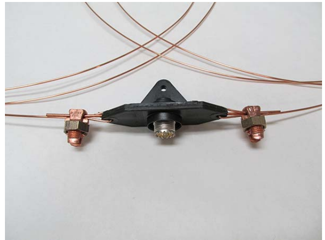
Detail of the center insulator. Split bolts need no soldering, for easy disassembly/reassembly later.
