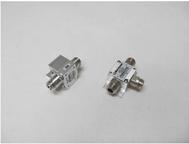
PolyPhaser surge arrestor and MiniCircuits power combiner. The surge arrestor is electrically bonded to the steel frame of the building where the feed line enters, which is in turn tied to a ground rod about 10' away. The power combiner is not grounded in my installation.
