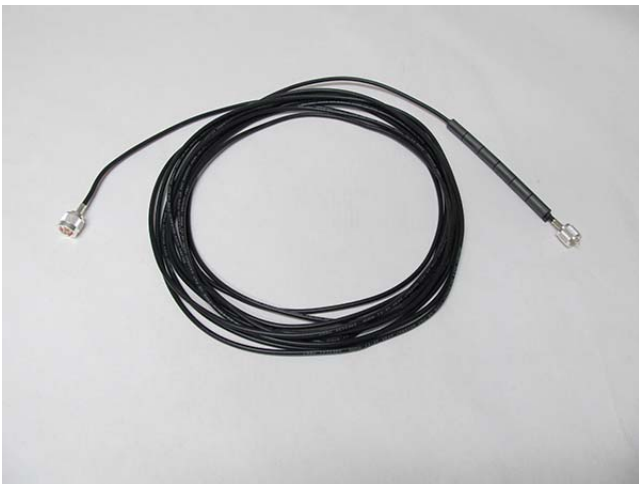
One piece of RG-58 (Belden 8259) cut to one wavelength long. The feed point end has a PL-259 crimp connector after six ferrite beads that form a common mode choke to act as a balun. The toroids fit snugly on the RG-58. The far end has an N-male crimp connector for the power combiner.
