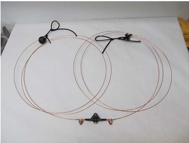
One of the two elements after pre-assembly. Small lengths of rope tied to end insulators make assembly in the field easy.
