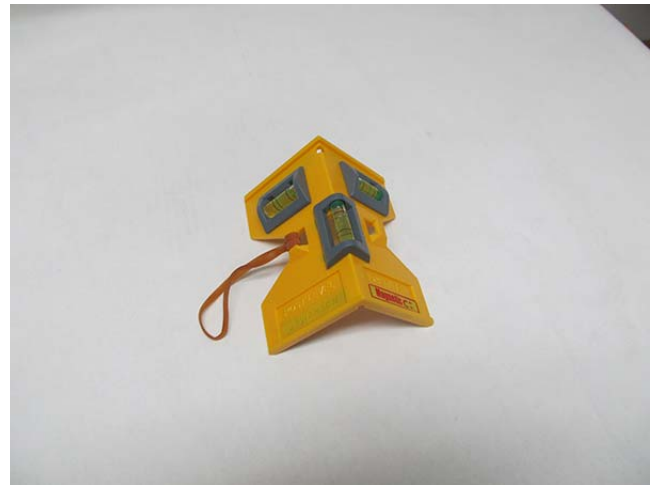
This wee four-dollar post level makes adjusting the guy lines a snap.
