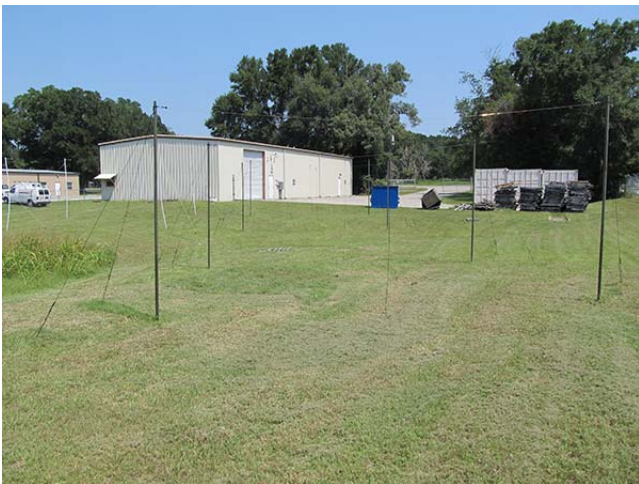
Looking north. Elements are supported by military surplus green fiberglass tent poles, three poles per mast, placing the elements 10' above the ground. Guy lines are 3/16" black polyester rope. With these materials, the array is quite stealthy and visually unobtrusive. All fixed ropes are tied with bowline knots; the adjustable guy lines are tied with trucker's hitches.
