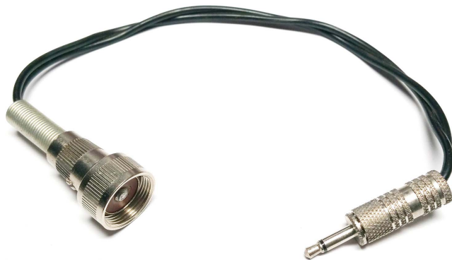
Figure 4 – Custom-made audio adapter cable. The male end on this cable is a mono (tip sleeve, or TS) 3.5 mm plug that happened to be on hand. The stereo (tip, ring, sleeve or TRS) equivalent is recommended to facilitate data acquisition from a second instrument on the second audio channel, if desired.
