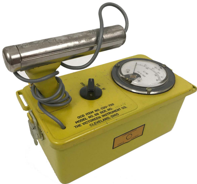
Figure 1 – The Victoreen CD V-700 Model 6B low range Geiger-Mueller survey meter.
