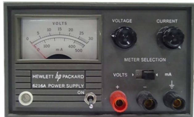
Figure 2 – The HP 6216A 0-30 VDC regulated power supply.
